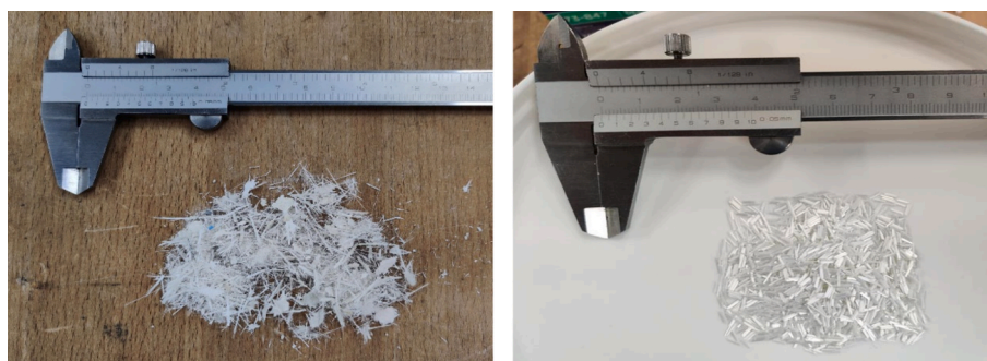
Fig. 1. Physical appearance of as-received SWTB (≤20 mm) (a) and as-received VF (b).
