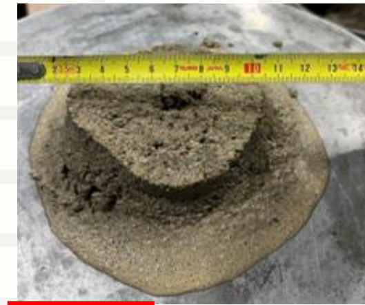
5% SWTB replaced mortar
