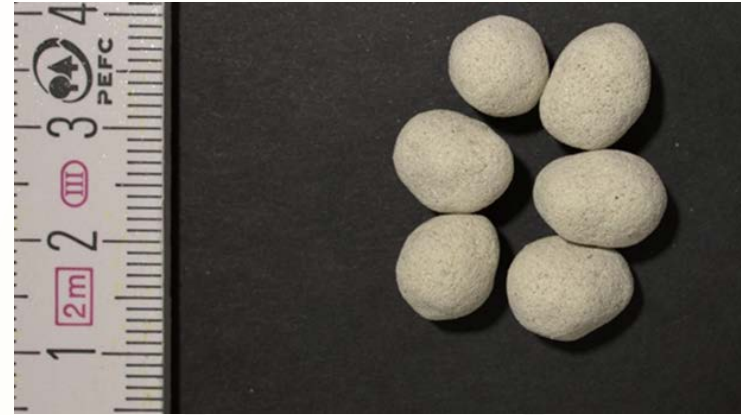
Pellets produced with cement and micro-sized SWTB particles
