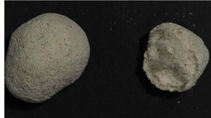
Pellets produced with cement and micro-sized SWTB particles
