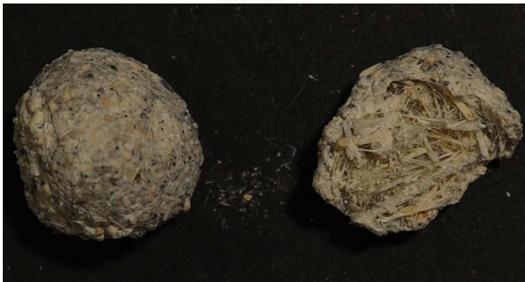
Pellets produced with cement and fibrous-granular SWTB waste
