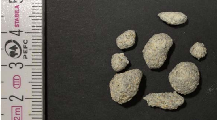
Pellets produced with cement and fibrous-granular SWTB waste
