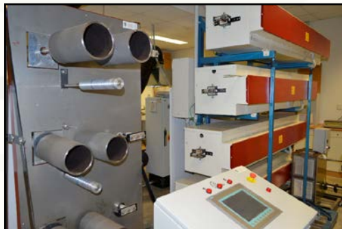
Continuous Carbonization plot line for CFs production
