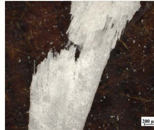
Flaws and irregularities on fiber cross-sections
