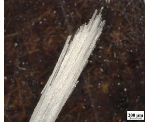
Optical microscopy image of shredded WTB
