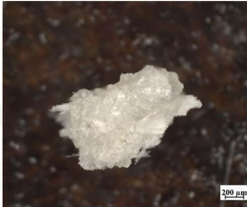
Optical microscopy image of shredded WTB
